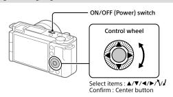
1 Set the ON/OFF (Power) switch to "ON" to turn on the camera.
